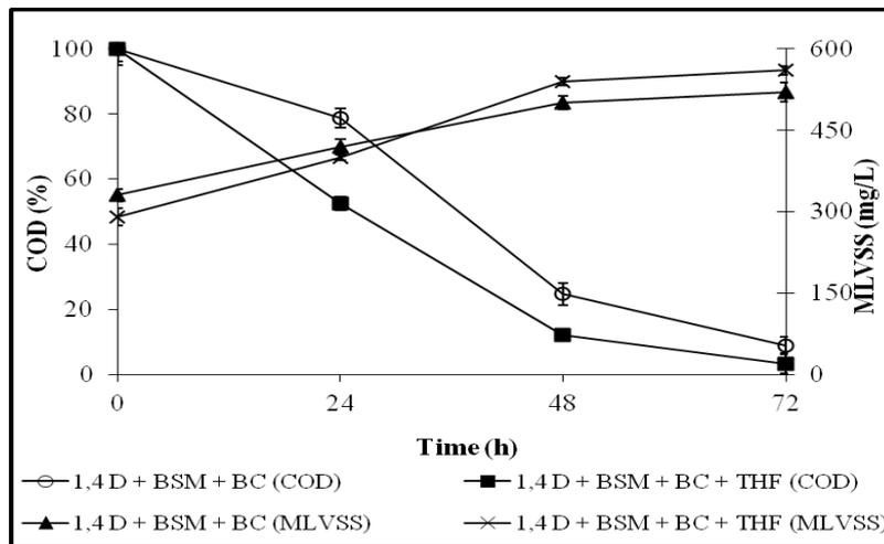
Fig. 6: COD and MLVSS profile during 1,4 dioxane biodegradation in the presence of THF
